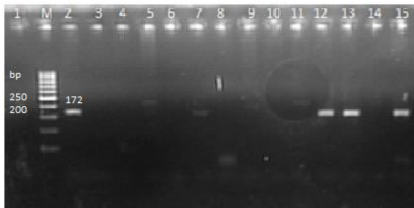
Figure 3. Gel electrophoresis of PCR products using ABI thermocycler device 1: Negative Control, M: DNA Marker (Leader 50 bp), 2,12,13,15: Positive cases (172 bp).
